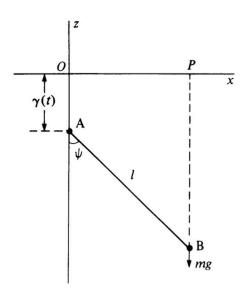
a mass m attached to a light, stiff rod AB of length l is free to move in a vertical plane. The end A of the rod is forced to move vertically, its distance from a fixed point O being a given function  $\gamma(t)$  of time. The mass is at point B. Refer to the figure for a schematic diagram of the system.
