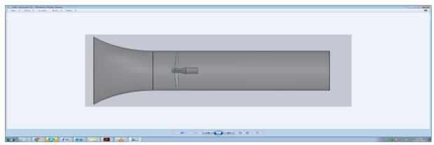
Ideal setup: Typical fan blade enclosed in duct with bell-mouth.
