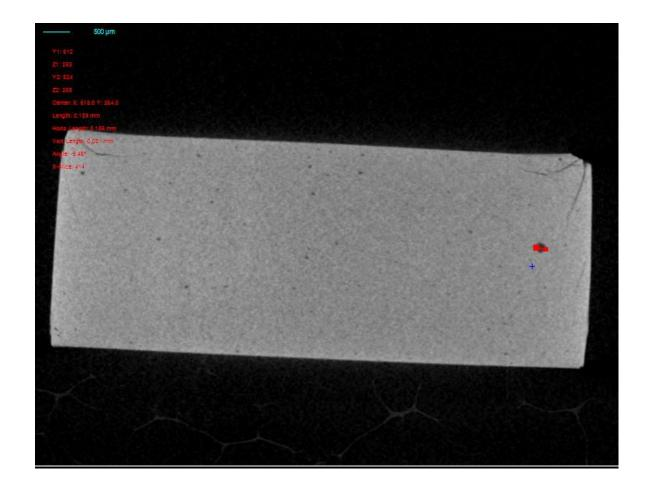
The aim of this study was to know the internal structure of the ceramic and to know about any defect/ impurities inside it. It is visible from the reconstructed images of top and front view that the sample has some holes. The largest hole is of the diameter 0.217 mm. the resolution of these images is 15.49 micron. It also has some cracks.
