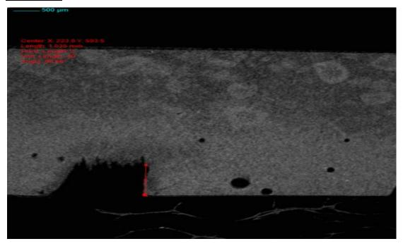
The objective of this study to know the dimension of the channel made on carbon composite and the deformation developed on the surface during manufacturing. A channel has been made using laser of 1 mm wide through the composite. It has been found in Computed Tomography (CT) study of this sample that the width of the channel is 0.941 mm which is
