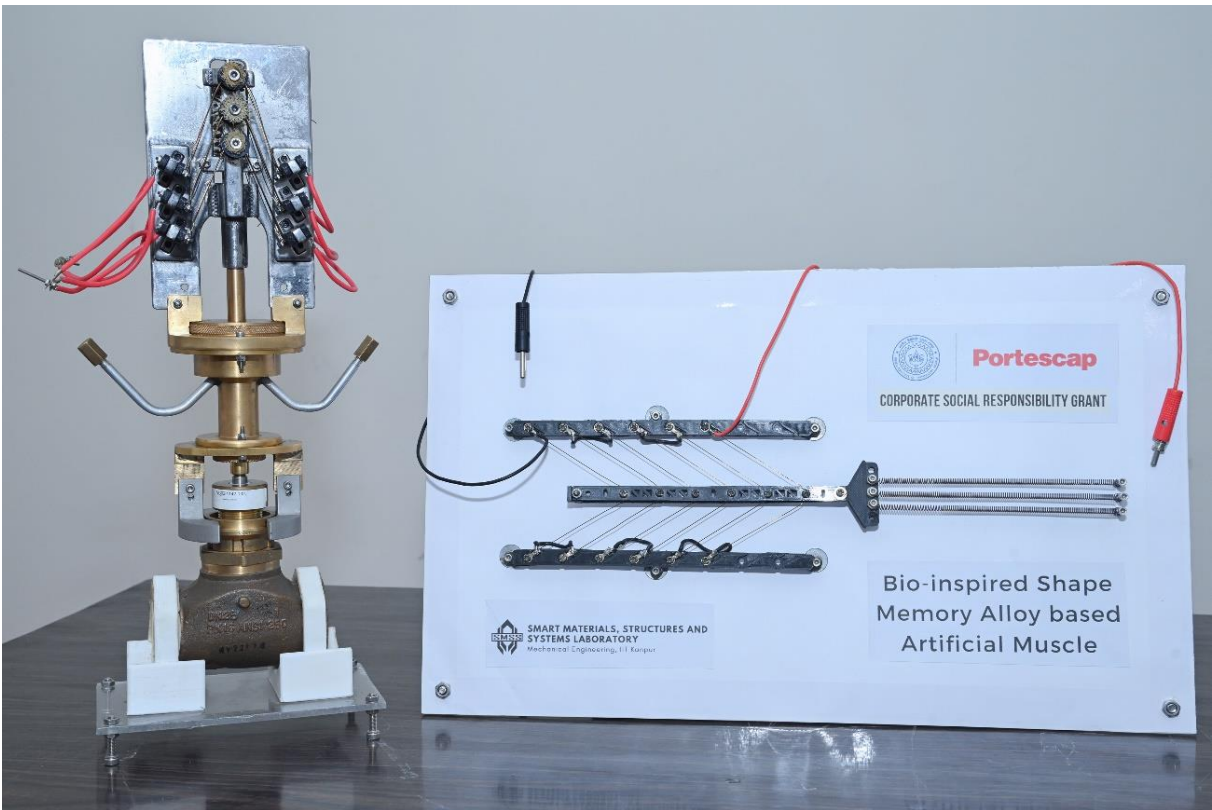
Figure #2: Design and development of non-magnetic hierarchical actuator powered by shape memory alloy based bipennate muscle.
