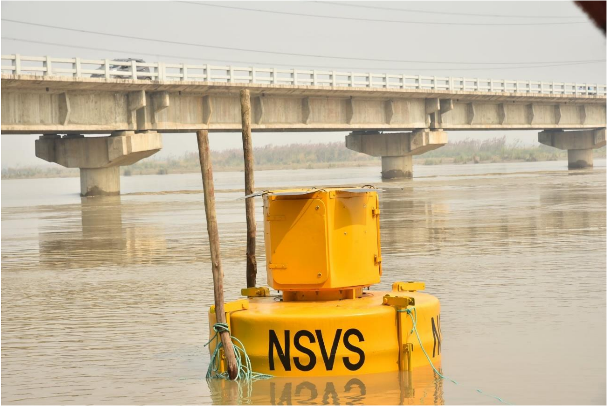
Figure #3: Design and Development of Aquatic Autonomous Observatory (Niracara Svayamsasita VedhShala - NSVS) for In situ Monitoring, Real Time Data Transmission and Web based Visualization.
