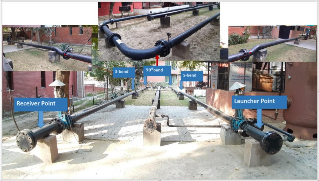
Figure #4: 8-inch pipeline test-bed facility with air compressor operational at Department of Mechanical Engineering, IIT Kanpur
