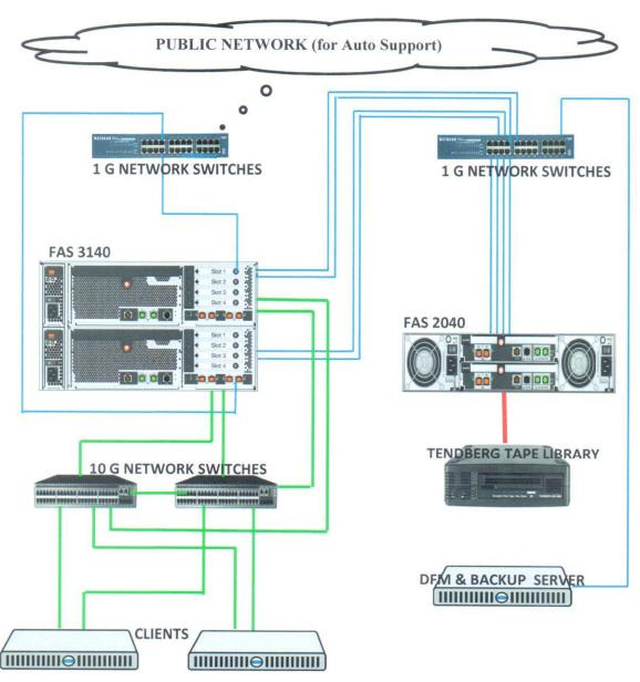
system. The current capacity of the primary storage is 25TB usable on RAID DP. Out of this 20TB is used by Linux based mailing systems and the remaining 5TB is used by the Exchange servers.
