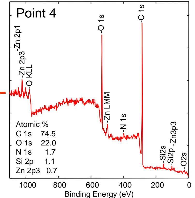
Spectrum obtained using 10 μm diameter x-ray beam detected Zn, probably Zn stearate
