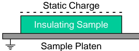
Traditional electron flood gun charge neutralization is not effective in neutralizing the localized positive charge created by the x-ray beam because the samples static charge interferes with the low energy electron beam.
