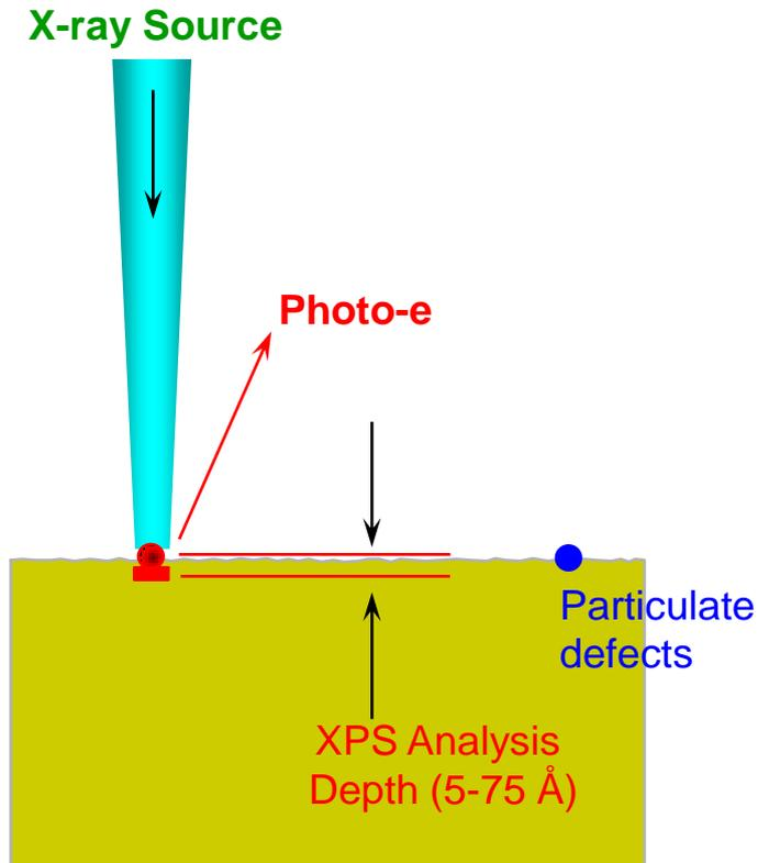
1. Only the generated photo-e from the top surface about 5 to 75Å can have enough energy to pop out of the sample surface.
